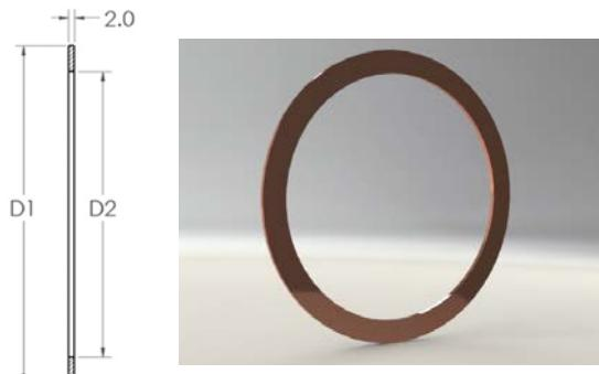
Oxygen free high conductivity (OFHC) copper is a suitable sealing material for bakeable UHV systems because of its good conformity with the thermal expansion coefficient of Stainless Steel as well as its essentially lower hardness (approx. 85 Brinell).
