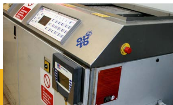
He leak test
