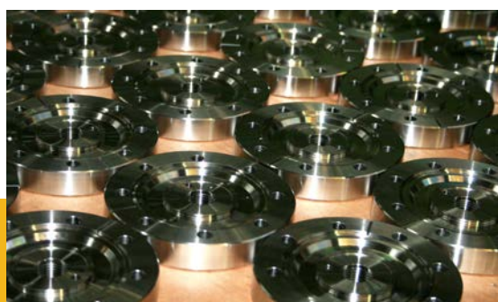
CF flanges after cleaning
