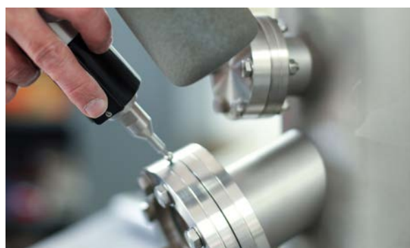
He leak test
