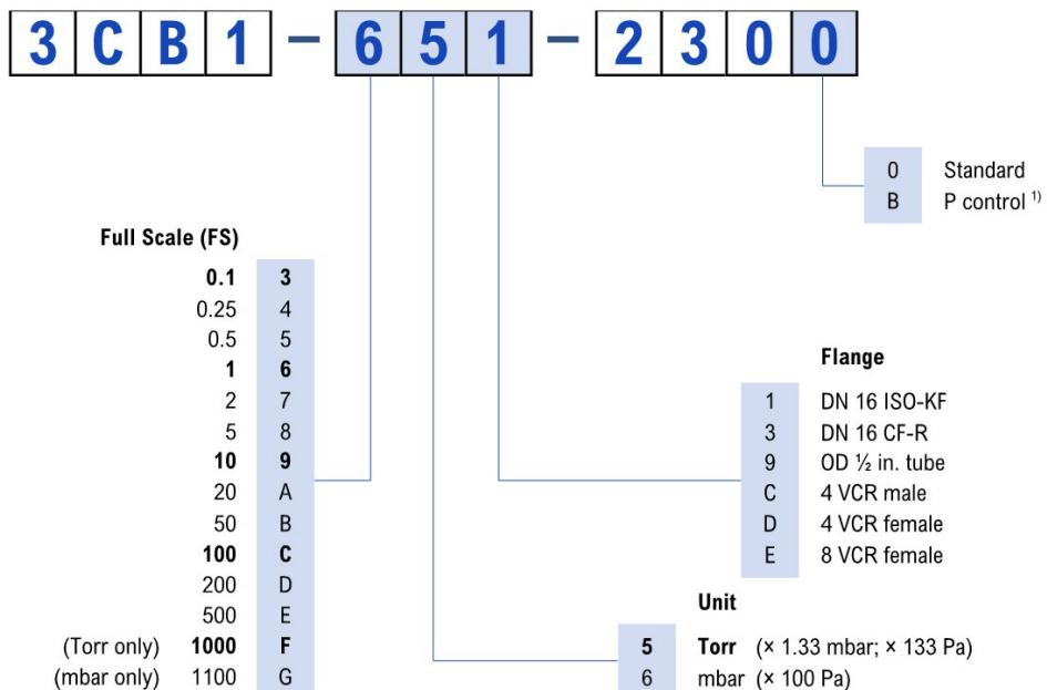
1) Optimized signal filter setting for pressure control
