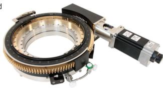
A preloaded ball bearing set accurately controls the rotating stage position. This allows the unit to be successfully used with manipulators and other precision positioning devices.
